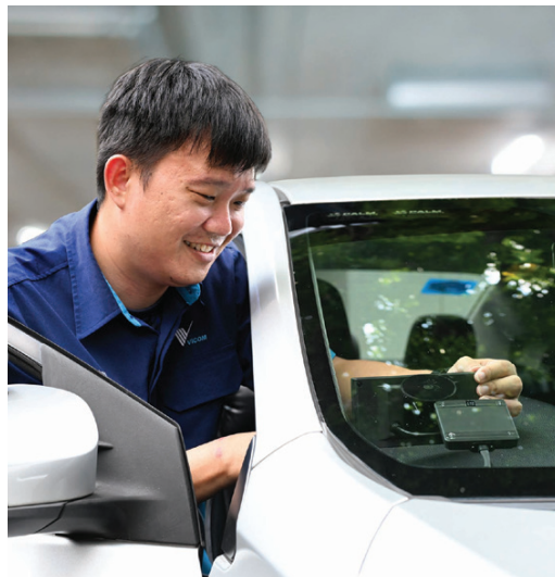
VICOM Inspector installing the new ERP 2.0 On-Board Units (OBUs).
